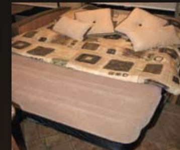
Cougar's sofa converts into an air mattress bed. The mattress is inflated/deflated by an electric pump. The bottom of the sofa serves as a storage drawer.
