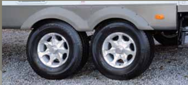
SIERRA's Aluminum Rims Provide You with Quality and Style. Rims come with E-Rated Radial Tires. (Standard Fifth Wheels)
