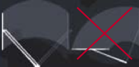
Pantographic windshield wipers (left) clean a wider swath of windshield than typical radial windshield wipers (right) of similar blade length.
